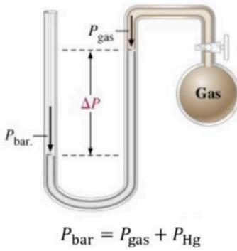
(c) Gas pressure less than barometric pressure
