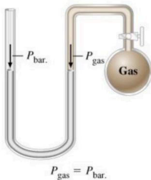
(a) Gas pressure equal to barometric pressure
