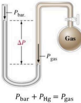
(b) Gas pressure greater than barometric pressure
